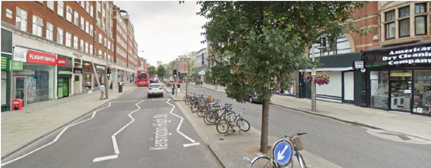
Kensington High Street, London (source: © 2018 Google). Central median supports informal pedestrian crossing movements, with cycling visually enforced. Staggered crossings replaced with straight over crossings.
